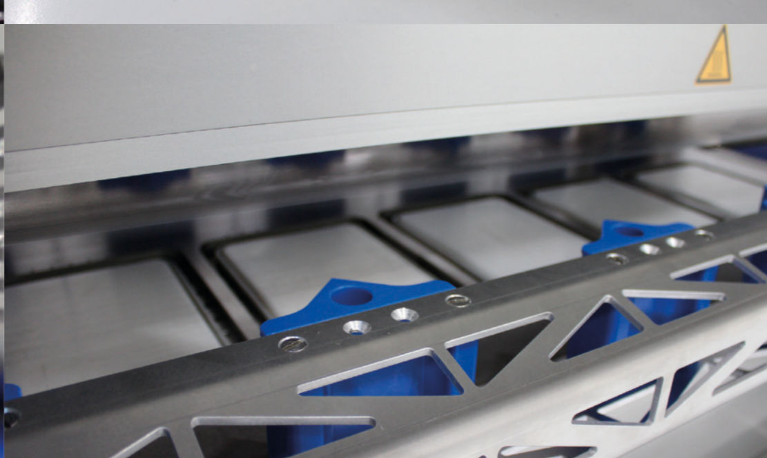
Gripper unit at sealing station
